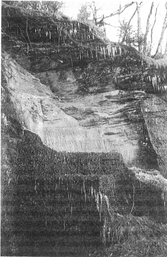
Figure 2: Part of the Öye greenschist quarry. The stone is sound when exposed (dark areas) and rather disintegrated when sheltered (light area).
