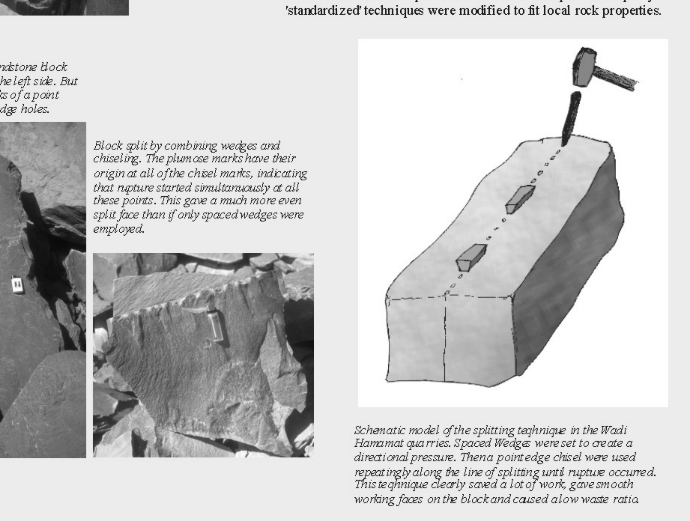
Schematic model of the splitting technique in the Wadi Hamamat quarries. Spaced wedges were set to create a directional pressure. Then a point edge chisel were used repeatedly along the line of splitting until rupture occurred. This technique clearly saved a lot of work, gave smooth working faces on the block and caused a low waste ratio.
